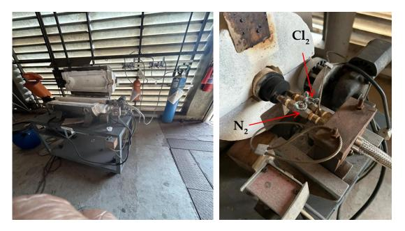
Figure 2- Reaction system used in lithium extraction tests from exhausted lithium-ion batteries.
