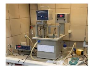
Figure 3: Reaction system used in the bio-extraction of base metals from electronic scraps.
