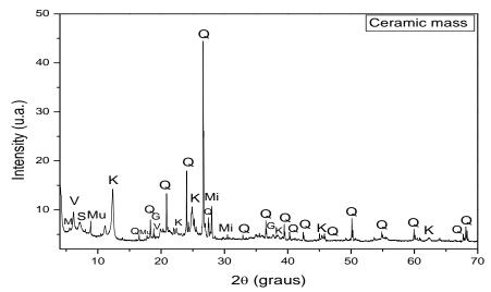
**Figure 3.** X-ray diffractogram of the ceramic mass. Q = Quartz, K = Kaolinite, M = Montmorillonite, G = Gibbysite, Mi = Microcline, Mu = Muscovite, S = Sepiolite, S = Sepiolite
