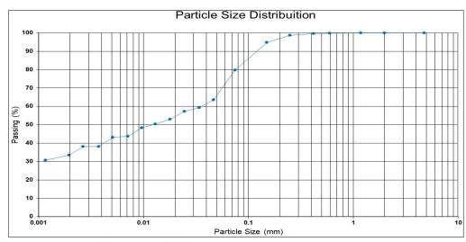
Figure 6. Ceramic mass particle size distribution.
