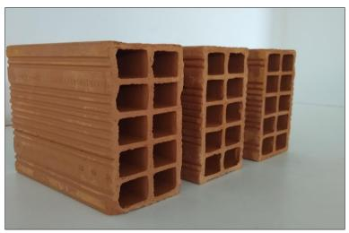
**Figure 2.** Sealing blocks with incorporation of 0%, 10% and 20% of wastes. **Source:** Prepared by the authors.
