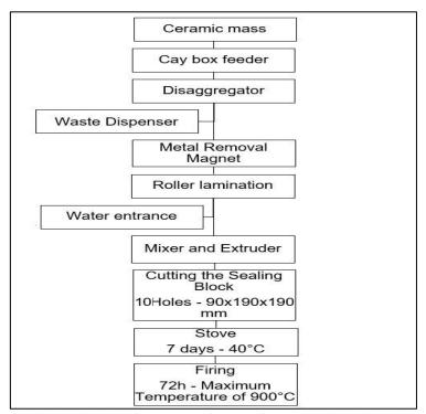
**Figure 1.** Flowchart of the industrial plant for the manufacture of red ceramic sealing blocks. **Source:** Prepared by the authors.
