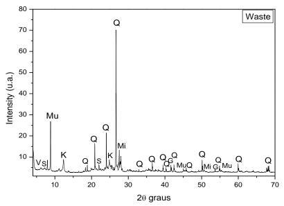
**Figure 4.** X-ray diffractogram of the waste. Q = Quartz, K = Kaolinite, G = Gibbysite, Mi = Microcline, Mu = Muscovite, S = Sepiolite, V = Vermiculite. **Source:** Prepared by the authors.
